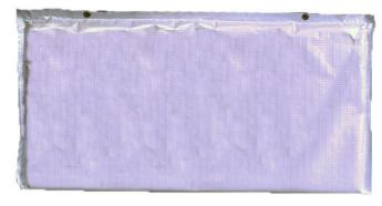
for standard duty incorporates a 1 ½" 1.6 lb. /cu. ft density fiberglass core. Type "B" features additional internal reinforcement at each grommet to withstand daily high pressure, hot water wash down in addition to a higher density (3lb. /cu. Ft.) 2" thick fiberglass core for improved acoustical performance.
